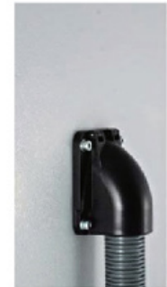
3. Lock FWS with screws
