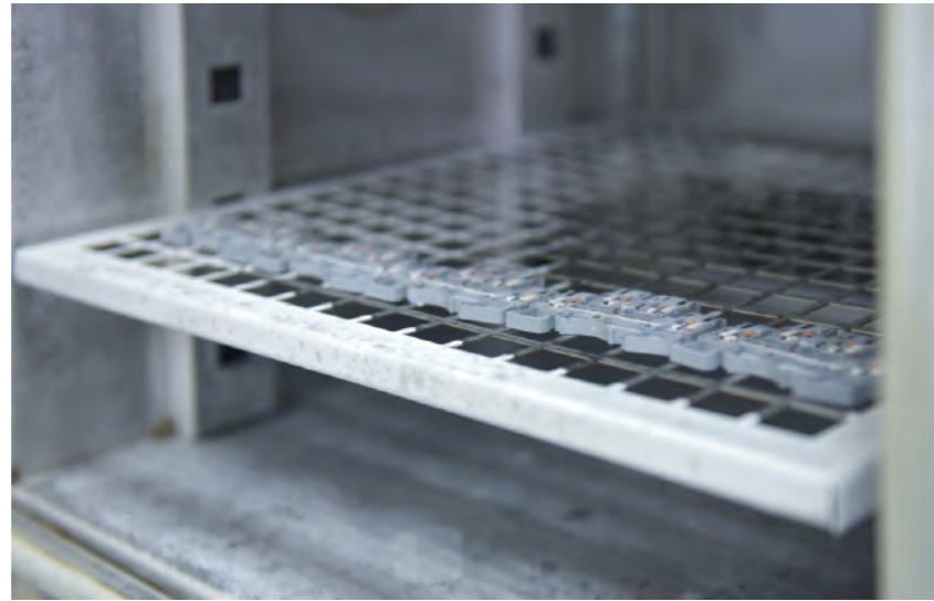
Din Rail Terminal Blocks Temperature Cycling Test
