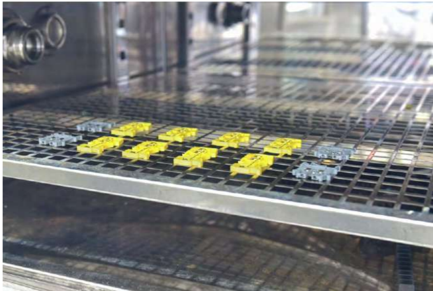
Din Rail Terminal Blocks Temperature Cycling Test
