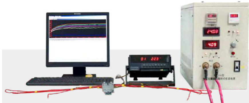
Din Rail Terminal Blocks Temperature-rise Test
